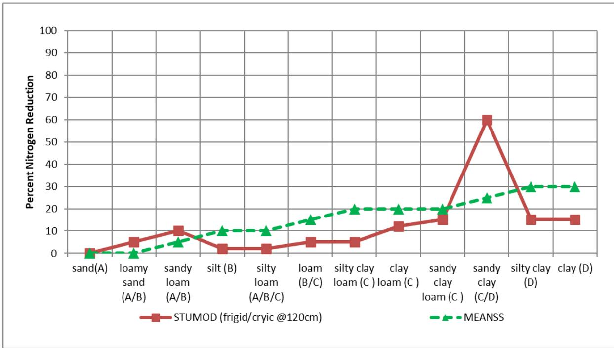
FIGURE 4. Comparison of STUMOD and MEANSS Nitrogen Reduction in Vadose Zone below the Drainfield.
