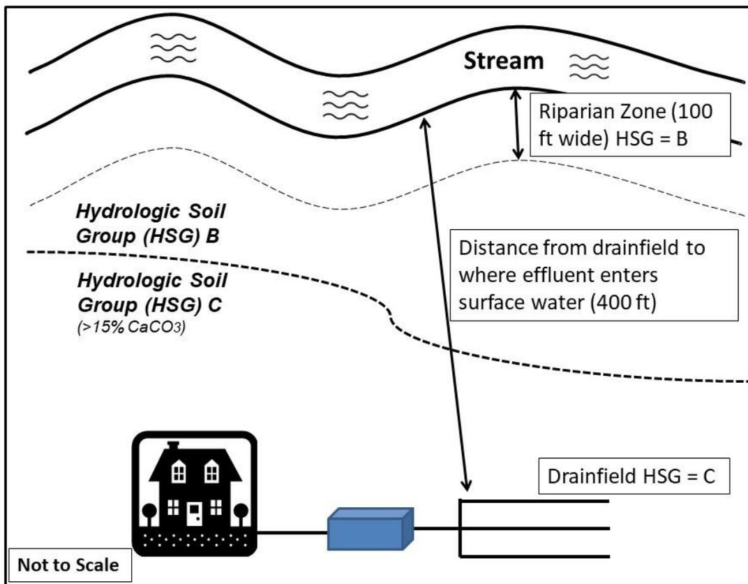
FIGURE 2. Plan view schematic of an example OWTS site showing MEANSS parameters, including hydrologic soil groups, distance to surface-water body, and riparian area.
